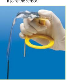
Continue pushing the sensor away from the closed, tight end of the sheath.
