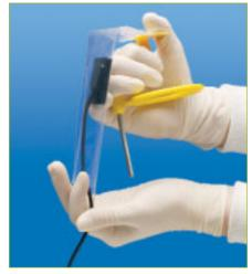
As the sensor is pushed into the wider area of the sheath, be careful to prevent the sensor from falling on the floor. Handle both sensor and cable gently.
